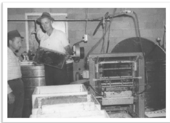
Photo 4. Dad showing extracted frame to queen breeder, Norm Rice, at a field day in the honey house in 1969. Davidson uncapper feeding two 21 frame Pender semi-radial extractors – state of the art then.
