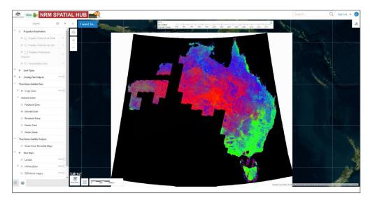
Figure 5. Area of fractional ground cover products generated from the entire 30yr Landsat archive.
